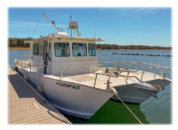
The power plants are Yanmar 6LPA-STP diesel engines driving Mercury Bravo IIX outdrives. Her cruising speed is 20-24 knots at 20gph while her WOT is 32 knots.
